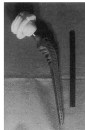
Fig. 4. Frialit Total Hip Replacement System: the cylindrical socket is made of the alumina ceramic as specified in the last column of Table 2. Its threads with asymmetrical cross section are designed for load transmission predominately by pressure. The BMO (biomechanically optimized) stepped stem is made of a TiAlFe alloy.
